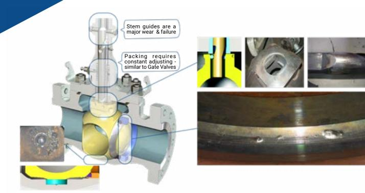
Traditional rising stem ball valves are prone to wear, high emissions, and frequent maintenance due to their linear motion and packing stress.
