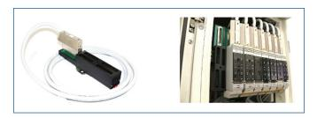
For FBM 200 series, field signals on termination assemblies are retained and the existing cable is replaced with a custom cable to route the signals to DeltaV I/O modules.
